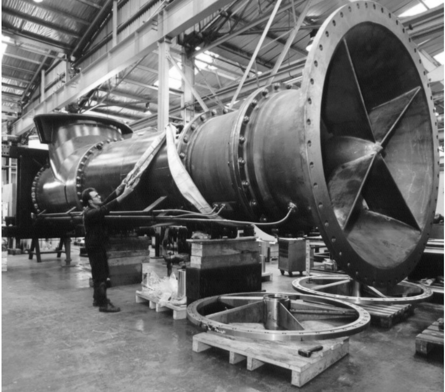
Semi-axial cooling water pump, Sulzer Pumps
